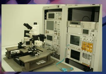
CLEANROOM FACILITY WITH RF MEASUREMENT AND ON-WAFER PROBE STATION. ADVANCED MEASUREMENT TOOLS FOR HIGH-FREQUENCY CIRCUIT TESTING.
